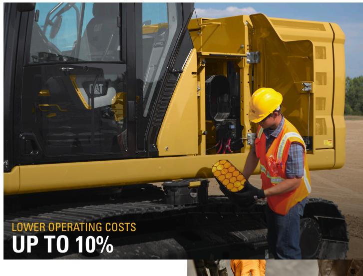
With extended and more synchronized maintenance intervals, you get more done at a lower cost. Consolidated filter locations make service faster. Hydraulic, air, and fuel tank filters have increased capacity and longer life.
